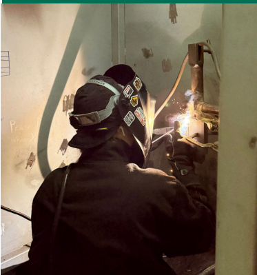
Brittany in the NMCC welding lab working on an unlimited vertical test, using 7018 rods.
